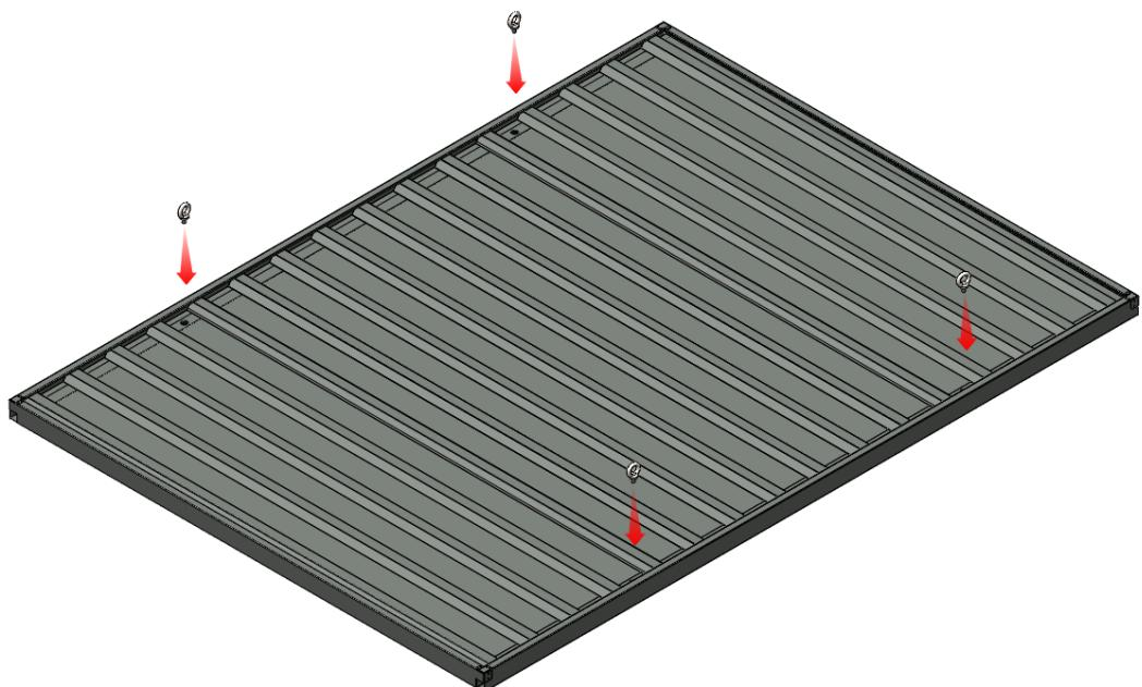
7- The roof panel is fastened to the adjacent panels with a pear-type spring pin.
