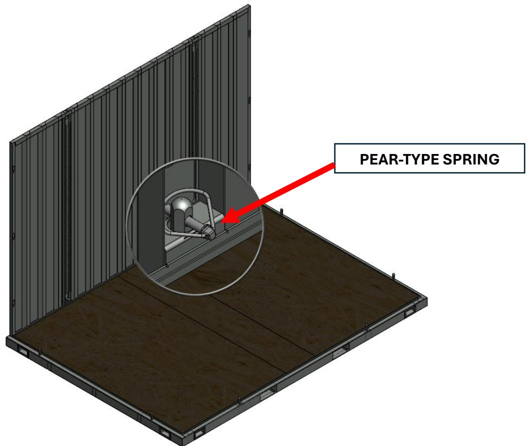
3- After the opposite side panel is mounted, it is secured with a spring pin.
