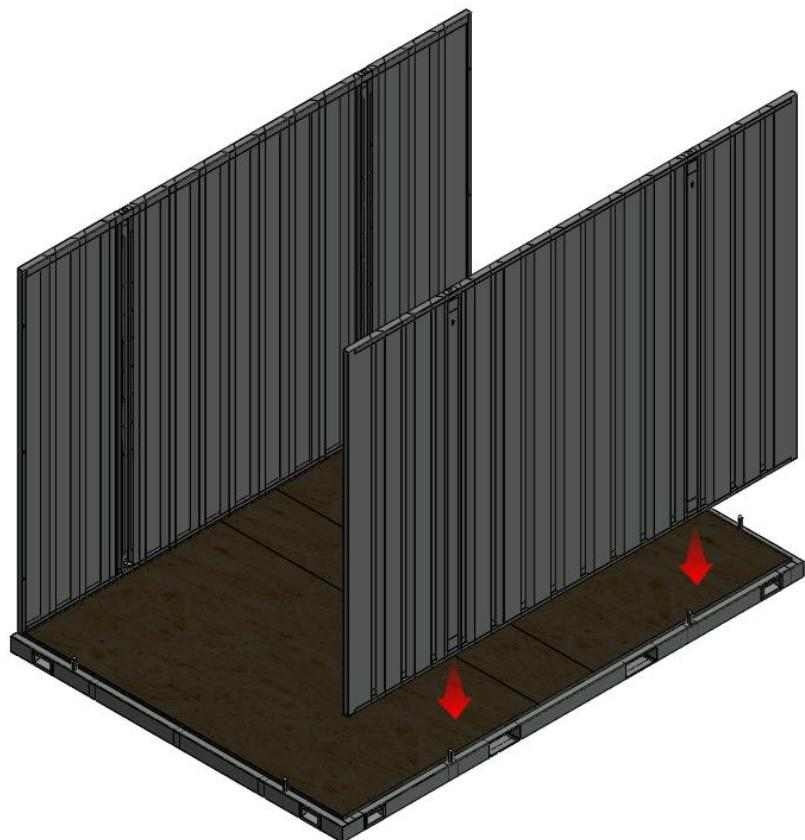
4- The front panel is installed and fixed to the chassis using a pear-type spring pin, and to the side panel using a D-type spring pin.
