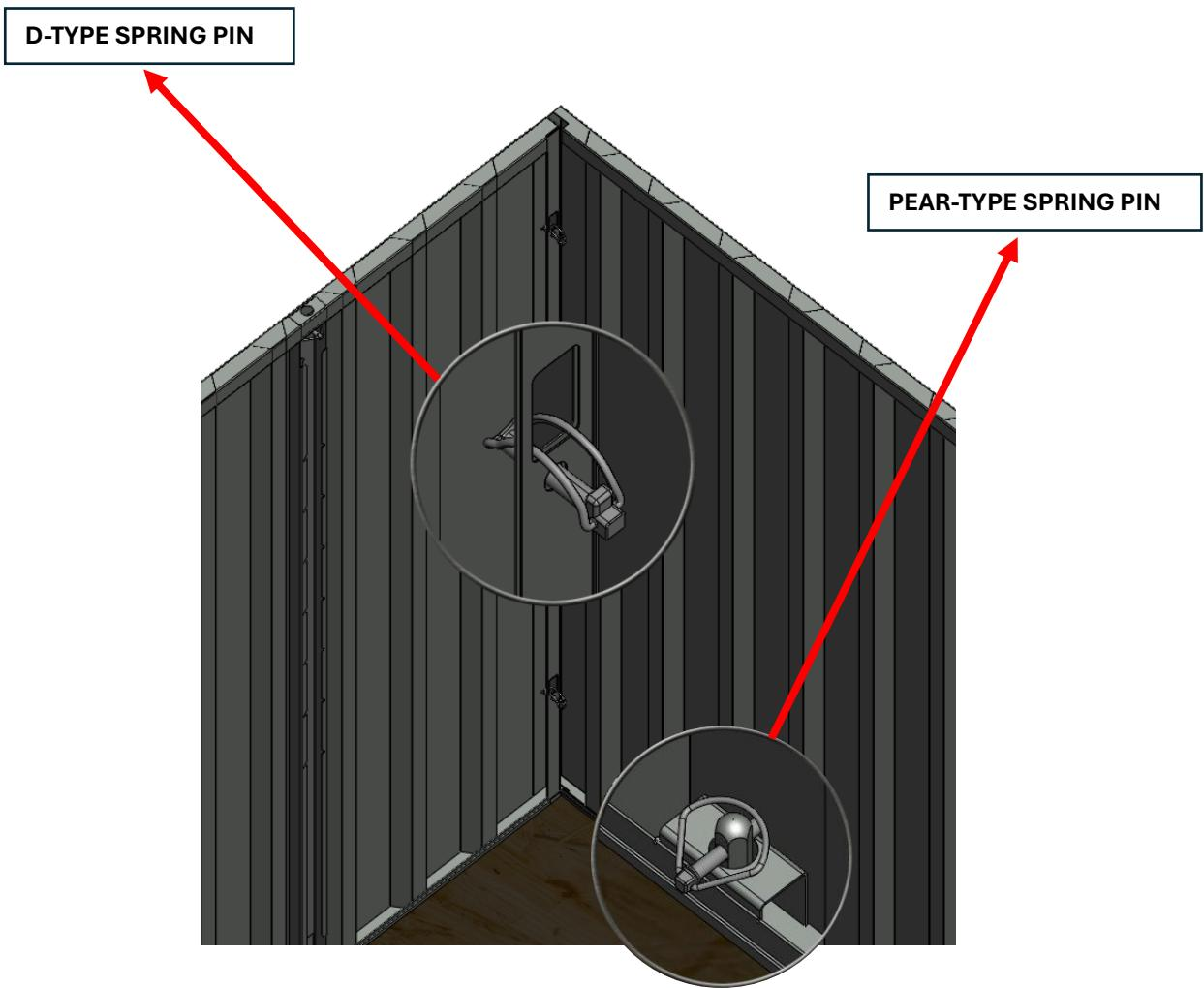
5- The door panel is mounted and fastened to the chassis using a pear-type spring pin, and to the side panel using a D-type spring pin.
